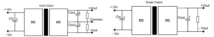
All the AM2LV-Z Series have been tested with the above recommended test circuit. This series should be tested under load.
