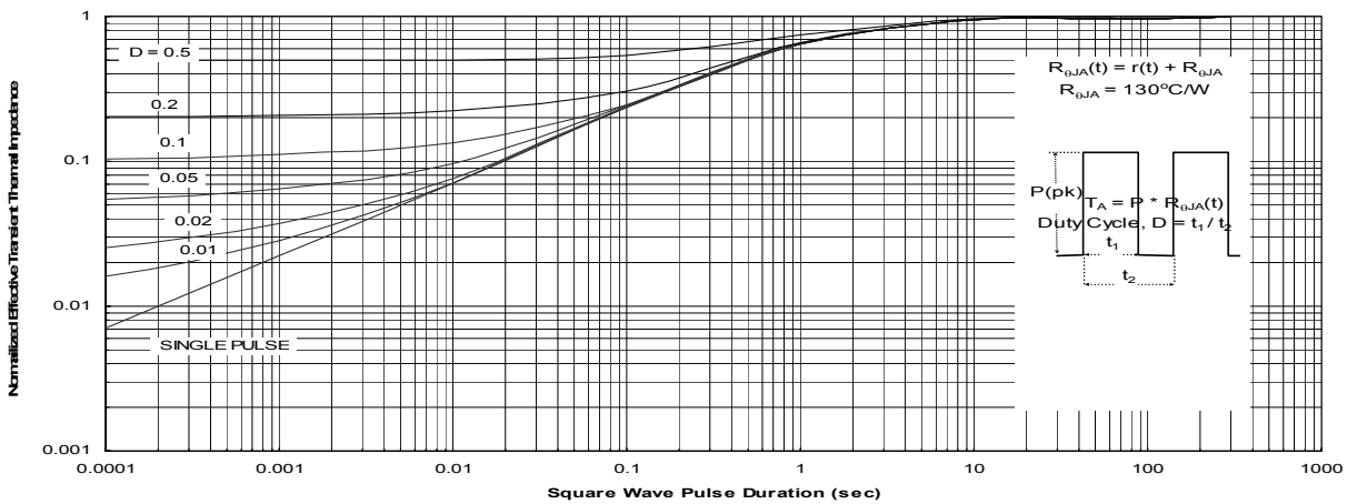
Normalized Thermal Transient Impedance, Junction-to-Ambient
