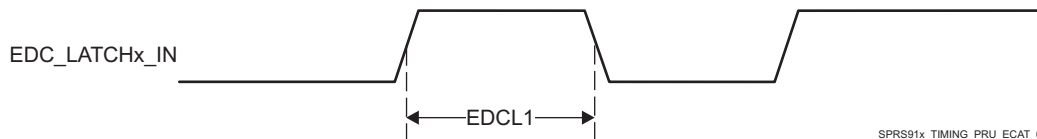
Figure 5-120. PRU-ICSS ECAT LATCHx_IN Timing
