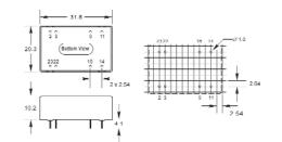
Note: All Pins on a 2.54mm pitch; All Pin diameters are 0.50 mm (Tolerance: $\pm 0.25$ ); All dimensions in mm.
