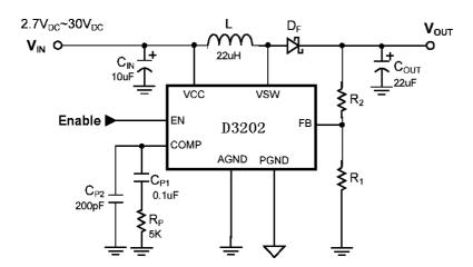
The AMC3202 develops a 1.276V reference from the FB pin to ground. Output voltage is set by connecting the FB pin to an output resistor divider and the maximum output voltage is determined by the VSW pin maximum voltage minus the output diode forward voltage. Referring to typical application circuit, the output voltage is set by the below formula(1):
