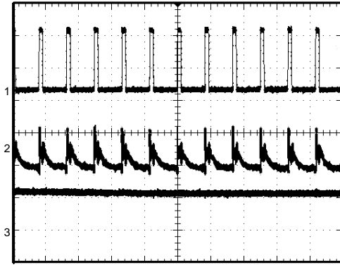
Typical Switching Waveform
