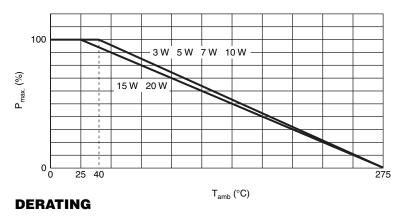
Maximum dissipation (P<sub>max</sub>) in percentage of rated power as a function of ambient temperature (T<sub>amb</sub>)
