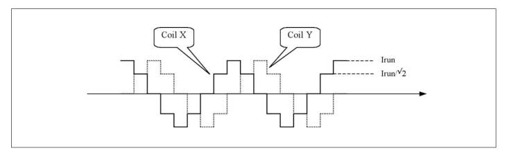
Whereas the figure below shows the current fed to one coil in 1/16<sup>th</sup> microstepping (1 electrical period).
