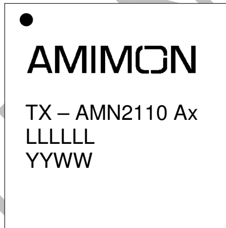
Figure 15: AMN2110 Package Marking
