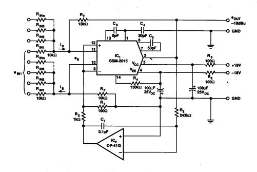
The output circuit topology of the SSM-2015 is complementary bipolar producing overall performance of  $6V/\mu s$  slew rate, and is able to drive a  $2k\Omega$  unbalanced load. The circuit described can be directly coupled, eliminating coloration and distortion associated with coupling capacitors. The circuitry following this amplifier could be AC (capacitor) coupled if the DC servo IC $_2$  offset voltage of  $\pm 10 mV_{DC}$  is objectionable.
