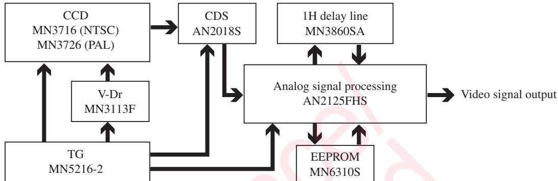
Note) The AN2125FHS can provide the analog CCD camera system without microcomputers.
