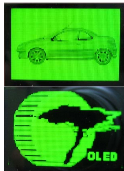
Figure 3. Example of Images on an OLED
