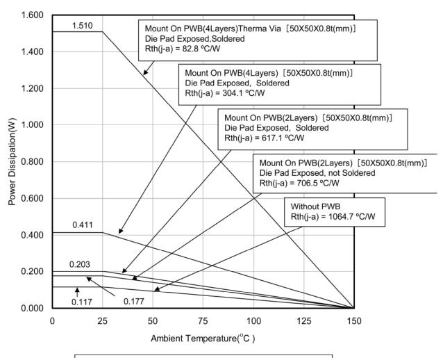
Mount On PWB(4Layers)Therma Via [50X50X0.8t(mm)] Die Pad Exposed,Soldered Rth(j-c) = 14.5 °C/W
