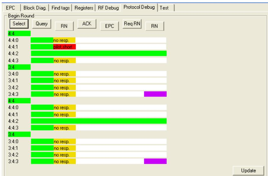
This tab is used to debug the EPC protocol using graphics. Details of communication required to execute one EPC operations *Inventory Round*, *Read*, and *Write* are shown. Rounds with slots and all EPC commands of communication are shown in color codes. Green color is used
