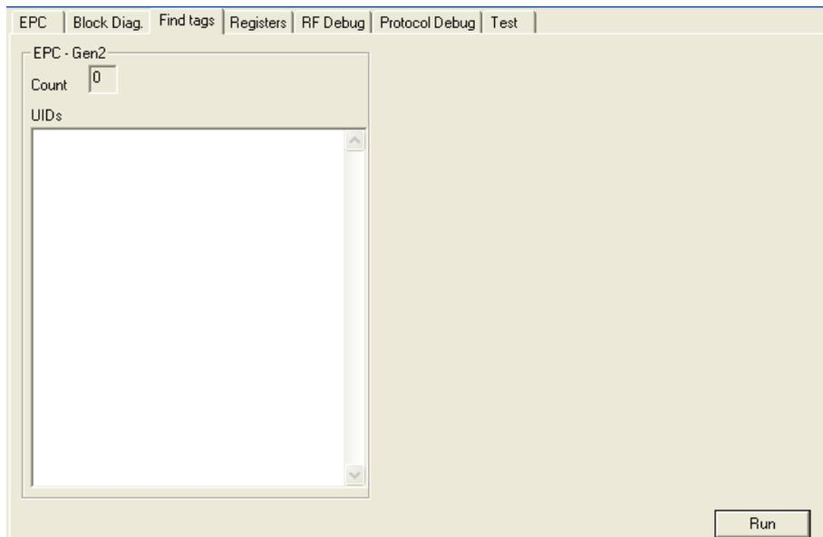
By changing into this tab, the active Reader is trying to identify all tags or labels in the RF field. The EPC numbers of the tags will be shown. This operation can be stopped and restarted with the **Stop / Run** button. No Reader to PC communication is echoed to the log window but it is still written to the log file (rfid-reader.log).
