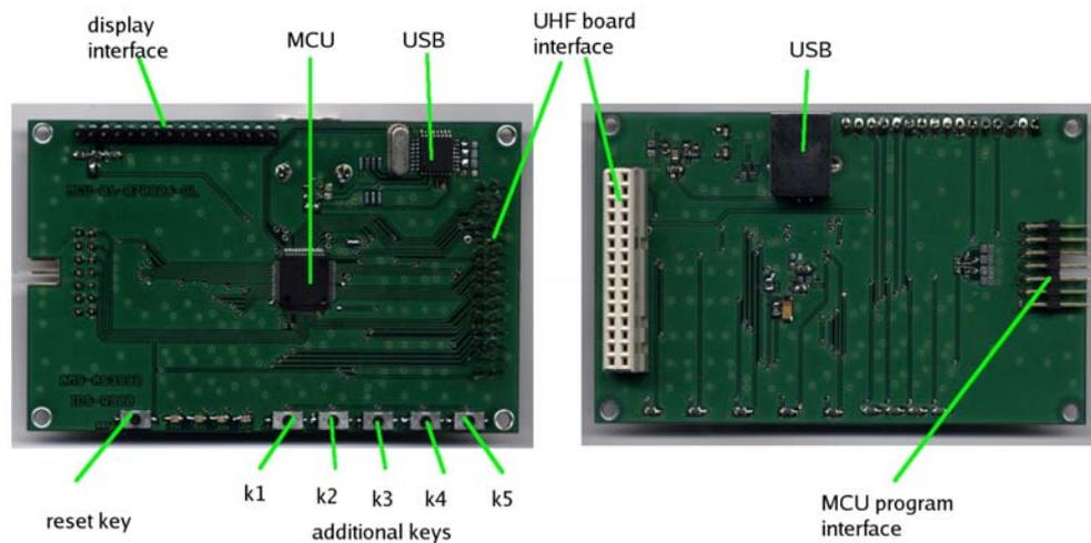
The MCU's reset can be done by reset key. Additional keys k4 and k5 are used for RF frequency setting while k1, k2, k3 are used for test purposes. The two boards are connected via 30 pin connector.
