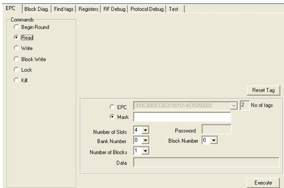
When this tab is activated only *Inventory Round* operation is enabled. You have to click **Execute** to run this operation and inventory the transponders before you can **Execute** other operations. When operations other than *Inventory Round* are selected modification of appropriate text entry and selection controls is enabled.
