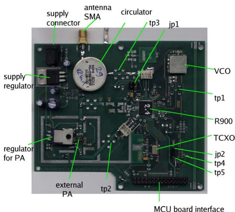
Two jumpers' jp1 and jp2 should be set for correct operation. Via the jp1 AS3990 is supplied and can be used for current consumption measurement. The jp2 is used to enable MCU support mode connecting the OAD2 pin to ground via 10k resistor (see details in the device specification).
