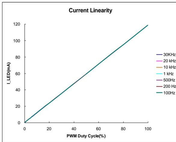
If the PWM pin remains low for longer than 32ms (i.e. the dimming frequency is well below 100Hz) the chip goes into a standby state. As soon as PWM goes H the chip executes soft start and resumes normal operation. This feature protects the system against high inrush current that could occur after a long idle period during which the output capacitor could be depleted of charge.
