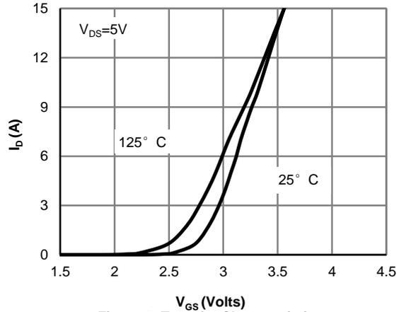
**Figure 2: Transfer Characteristics**
