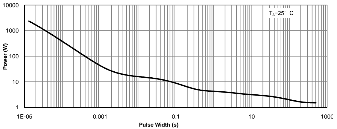
Figure 11: Single Pulse Power Rating Junction-to-Ambient (Note F)
