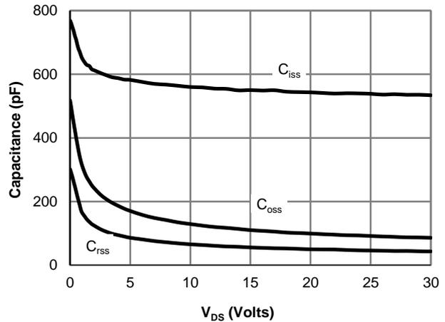
**Figure 8: Capacitance Characteristics**
