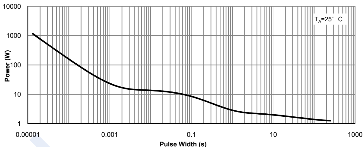
Figure 11: Single Pulse Power Rating Junction-to-Ambient (Note F)
