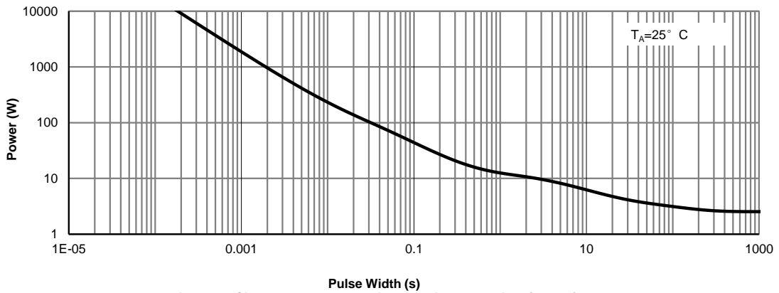
Figure 14: Single Pulse Power Rating Junction-to-Ambient (Note H)
