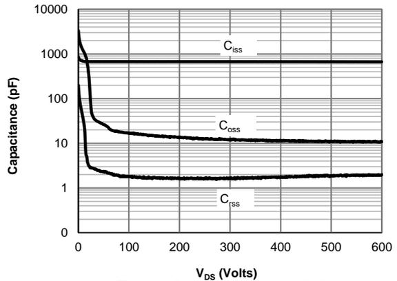
**Figure 8: Capacitance Characteristics**
