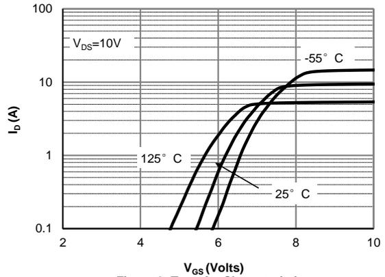
**Figure 2: Transfer Characteristics**
