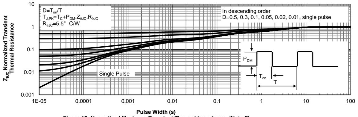
**Figure 12: Normalized Maximum Transient Thermal Impedance (Note F)**
