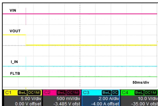
Figure 15. Short Circuit Protection (No Load, Device Option -04)
