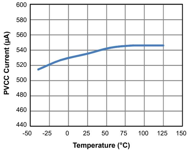
Figure 5. Supply Current ( $I_{VCC}$ ) vs. Temperature
