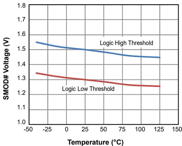
Figure 7. SMOD# Threshold vs. Temperature
