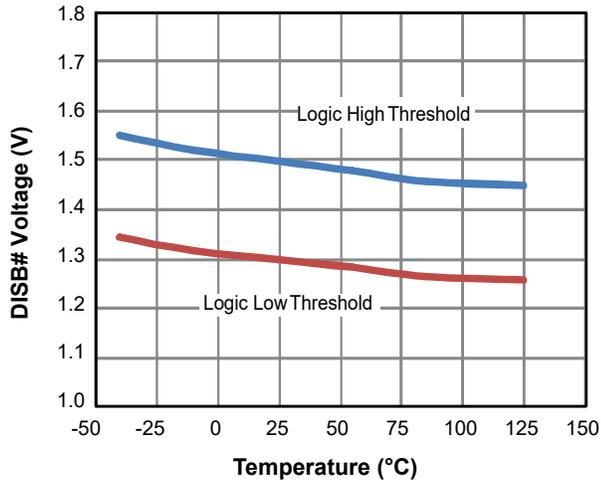
Figure 9. DISB# Threshold vs. Temperature
