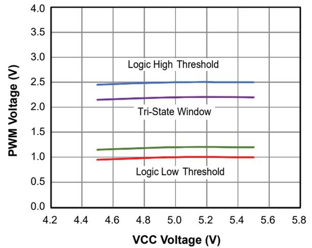
Figure 10. PWM Threshold vs. VCC Voltage
