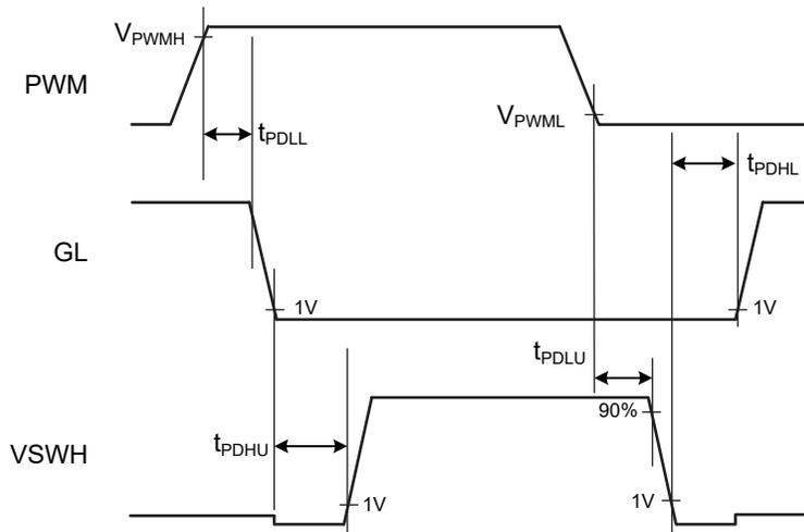
Figure 1. PWM Logic Input Timing Diagram
