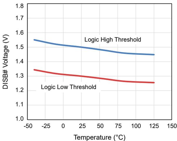
Figure 7. DISB# Threshold vs Temperature
