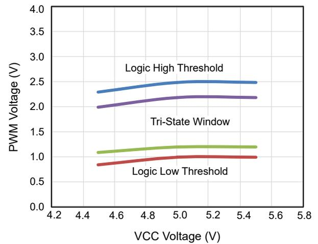
Figure 8. PWM Threshold vs VCC Voltage
