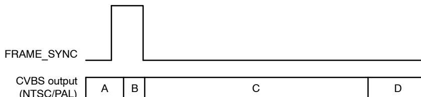
Figure 9. Frame Sync Behavior with Interlaced Mode
