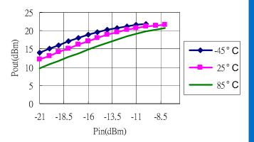
Pout v.s. Pin Biased at 5V
