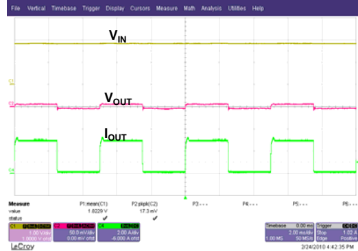
Load Transient (Sink test)
