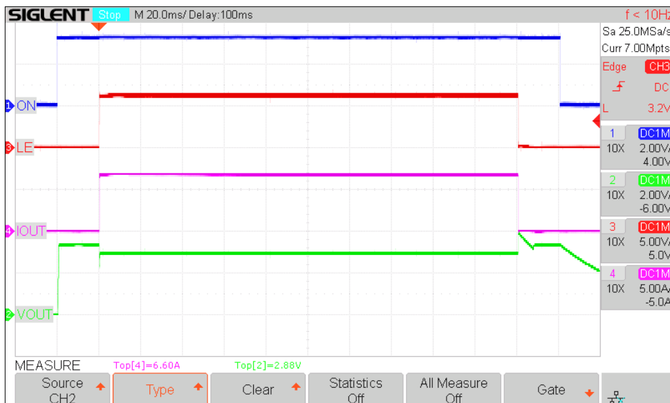
Figure 10. AP220309 ACL Operation Waveform. V_{DD} = V_{IN} = 3.3V , R_{LOAD} = 20\Omega , C_{OUT} = 10\mu F , C_{SLEW} = 3.9nF . Load Enable signal applies additional 0.4\Omega of load.
