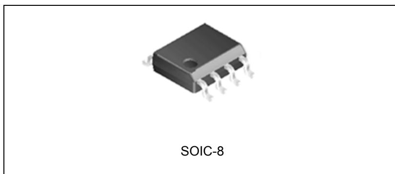
Figure 1. Package Type of AP3502F
