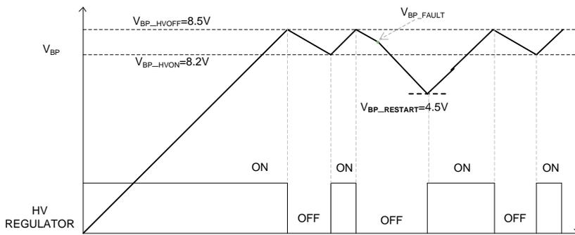
Figure 1. V<sub>BP</sub> Waveform and HV Regulator ON/OFF Status
