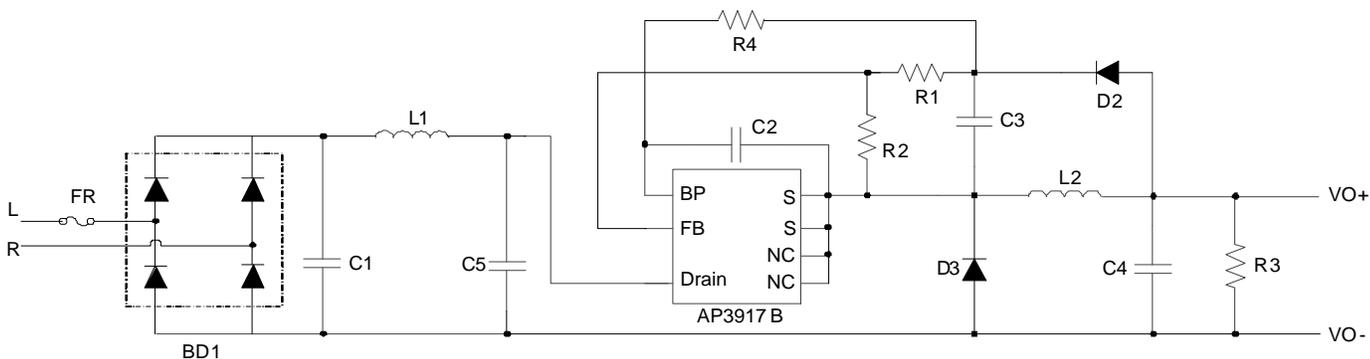
Figure 2. Low Standby Power Circuit with Auxiliary V<sub>BP</sub> Supply
