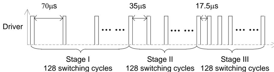
Figure 4. Driver Time Sequence in Startup Process
