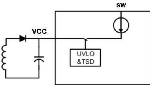
Fig 1 Startup circuit
