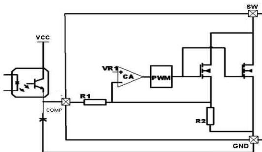
Fig 2 Feedback Circuit
