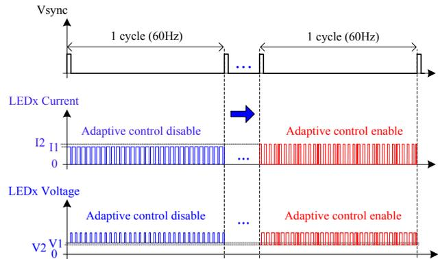
Figure 5: Adaptive Control Mode Example
