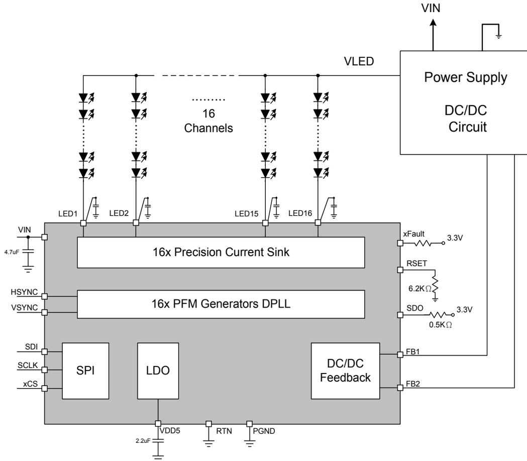
Note: When LED1 to 16 of APE5030A pin-out location to external LED string cathode location has exceeded 1uH wire inductance, suggestion add the MLCC capacitors for holdout interference.
