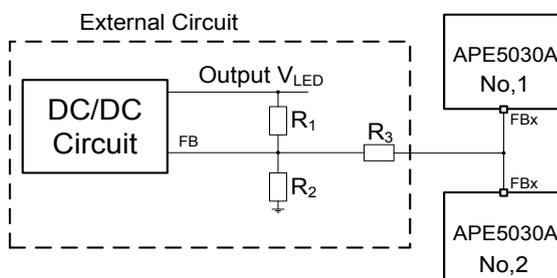
If possible; try to let FBx pin terminal keep to 0.25V and it's not less than 0.25V.
