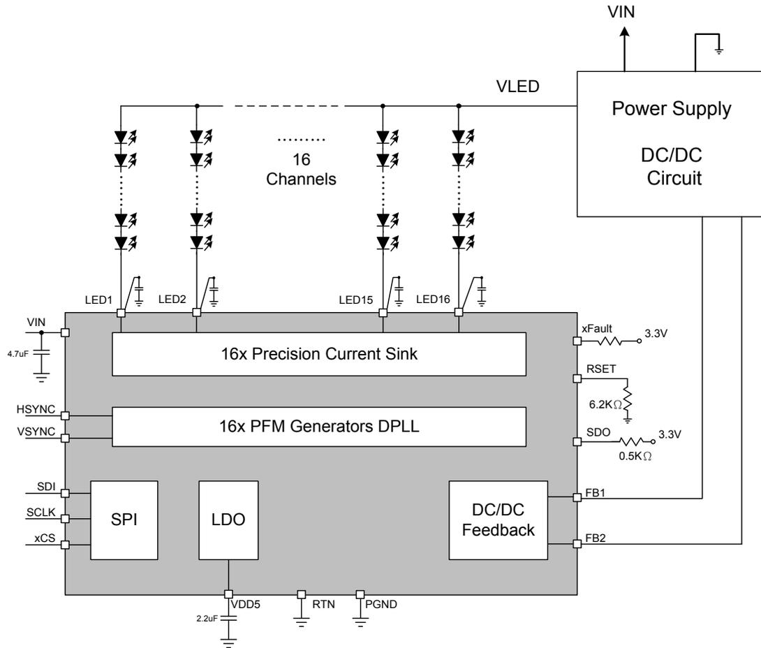
Note 4: When LED1 to 16 of APE5030A pin-out location to external LED string cathode location has exceeded 1uH wire inductance, suggestion add the MLCC capacitors for holdout interference.
