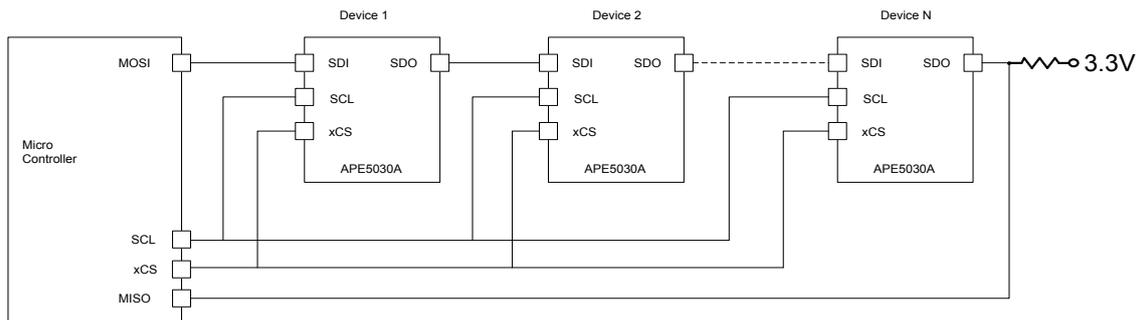
Figure 7: SPI Daisy Chain structure
