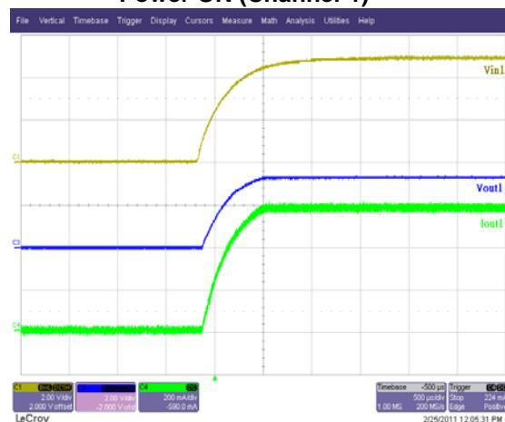
$V_{IN1}=5V$ ,  $V_{OUT1}=3.3V$ ,  $I_{OUT1}=600mA$
