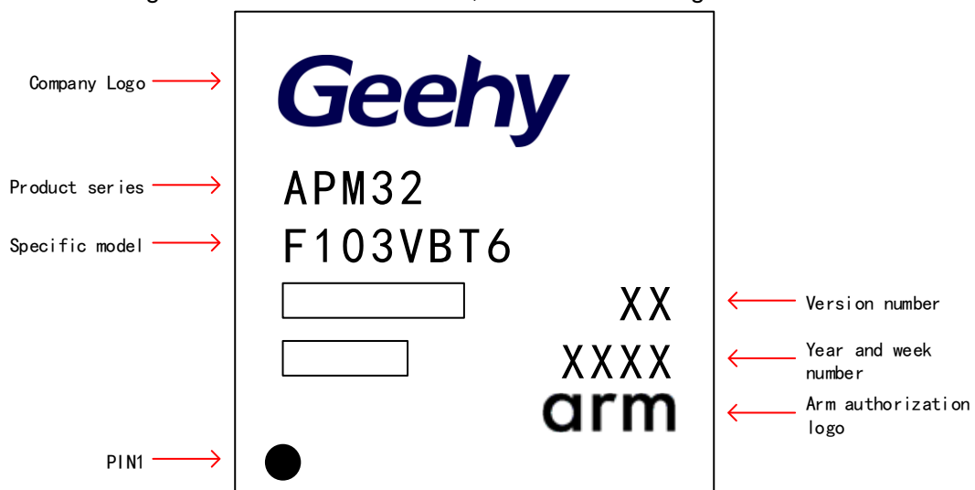
Figure 22 LQFP100 - 100 Pins, 14 x 14mm Package Identification
