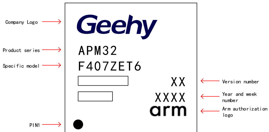
Figure 22 LQFP144 -144 Pins, 20 x20mm Schematic Diagram
