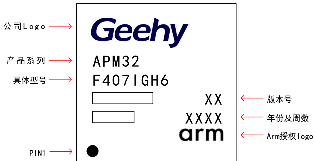
图 31 LQFP64 - 64 Pins, 10 x 10mm Package Schematic Diagram
