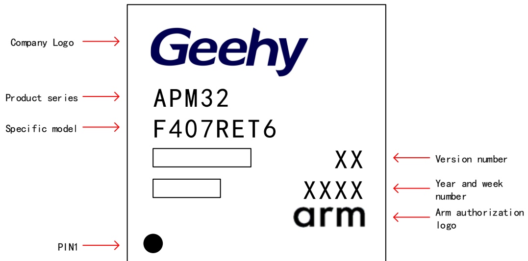
Figure 28 LQFP64 - 64 Pins, 10 x 10mm Package Schematic Diagram
