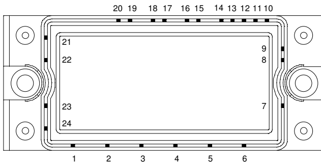
APTGS10X120RTP2: Without Brake (Pin 7 & 14 not connected)
