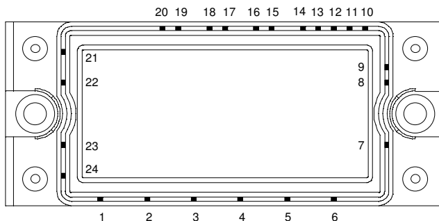
APTGS25X120RTP2: Without Brake (Pin 7 & 14 not connected)
