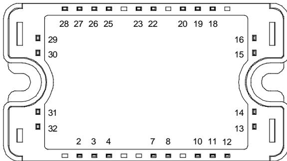
All multiple inputs and outputs must be shorted together
