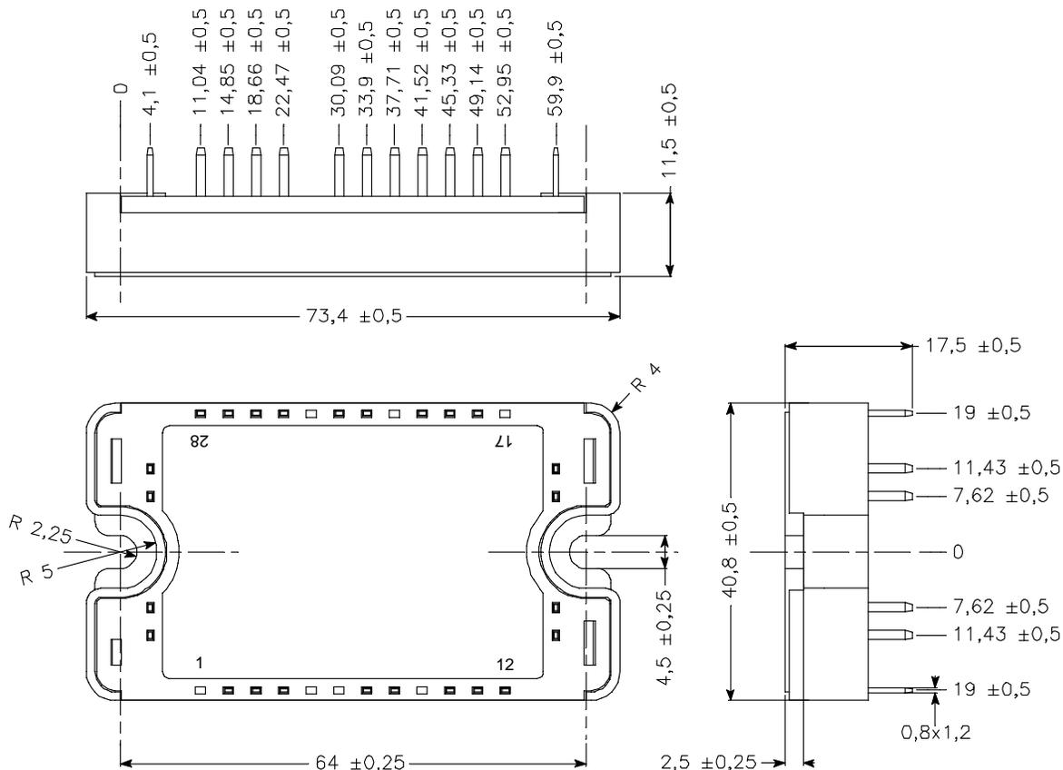
See application note 1901 - Mounting Instructions for SP3 Power Modules on [www.microsemi.com](http://www.microsemi.com)
