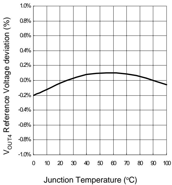
Note : The Reference Voltage( $V_{REF}$ ) Deviation is  $\frac{V_{REF}(T_J) - V_{REF}(25^{\circ}\text{C})}{V_{REF}(25^{\circ}\text{C})} \times 100\%$
