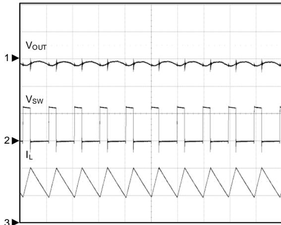
CH1:  $V_{OUT}$ , 50mV/Div, DC
