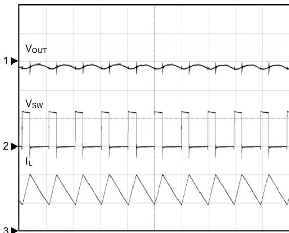
CH1:  $V_{OUT}$ , 50mV/Div, DC
