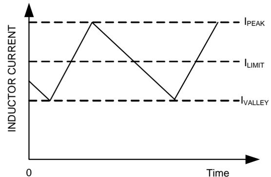
Figure 2. Current Limit Algorithm
