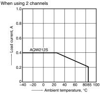
1.-(2) Load current vs. ambient temperature characteristics
