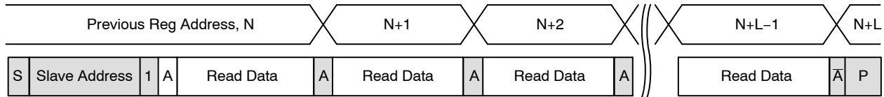
Figure 40. Sequential READ, Start from Current Location
