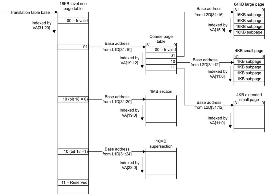
**Figure 5-5 Backwards-compatible section, supersection, and page translation**
