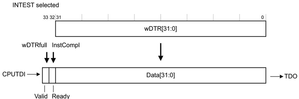
**Figure 13-10 Scan chain 5 bit order, INTEST selected**
