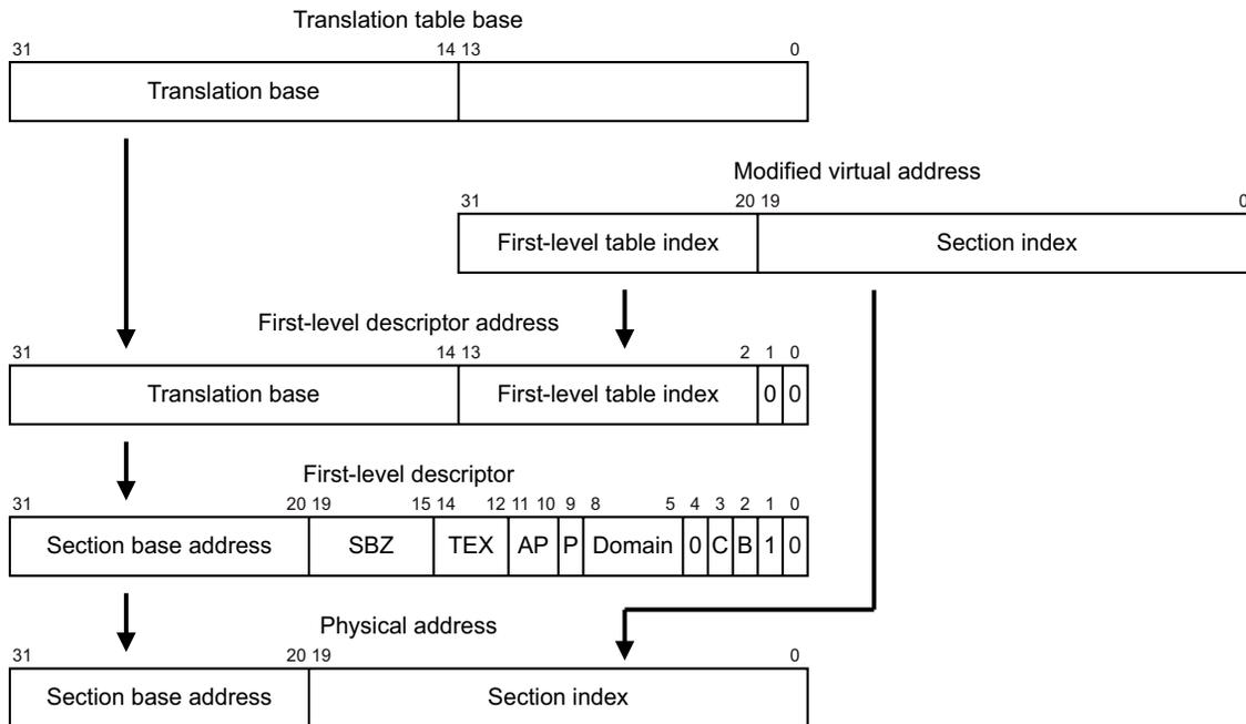
**Figure 5-12 Translation for a 1MB section, backwards-compatible format**
