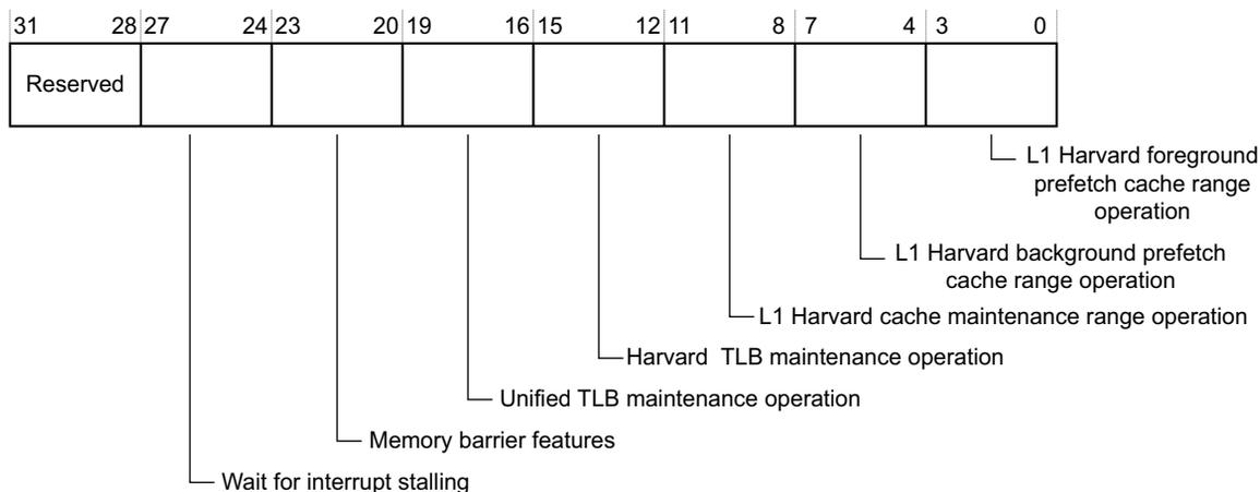
**Figure 3-11 Memory Model Feature Register 2 format**
