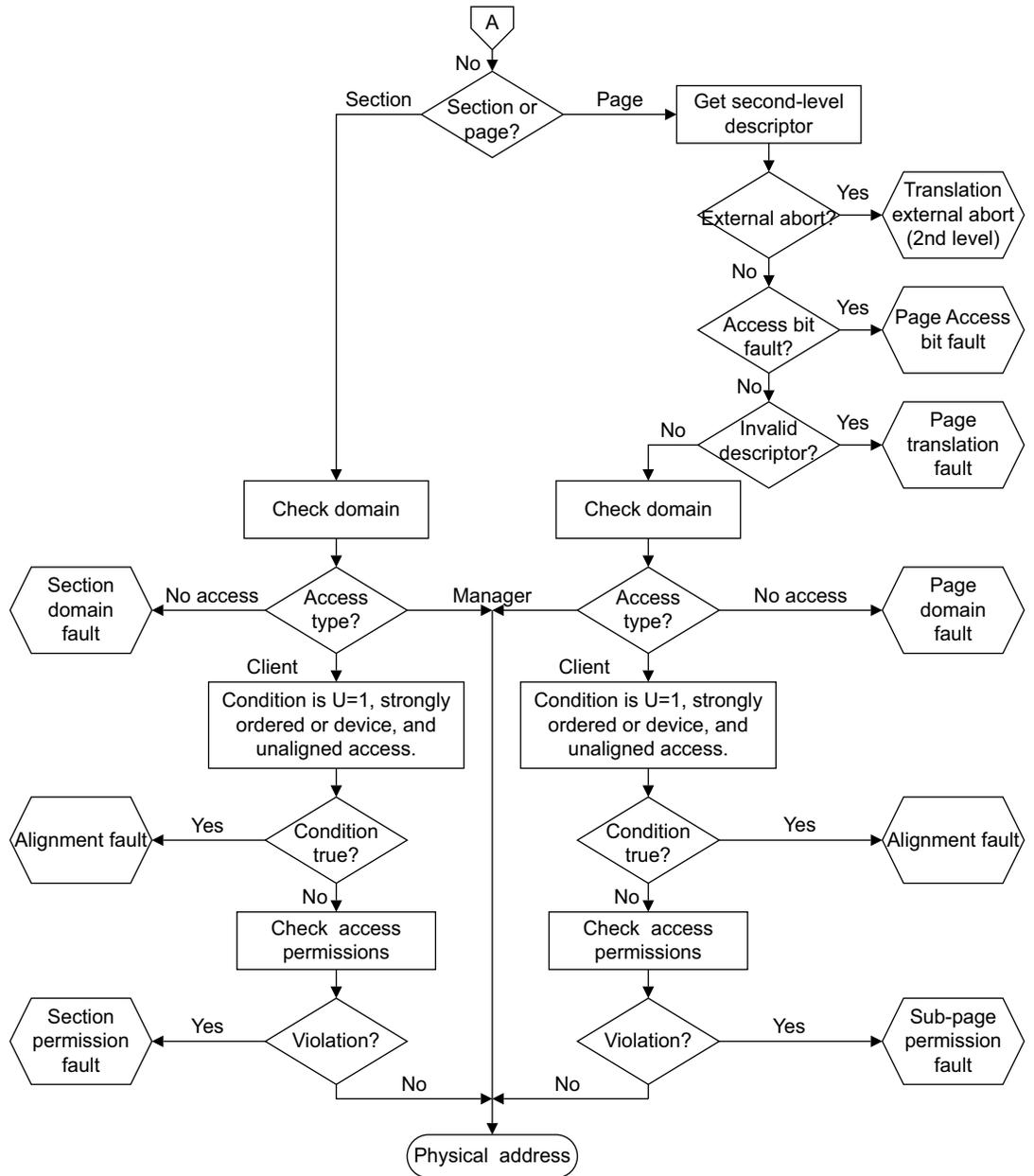
Figure 5-2 Translation table managed TLB fault checking sequence 2
