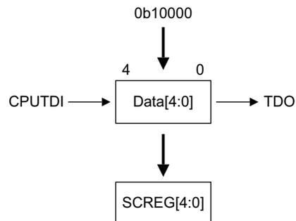
Figure 13-5 Scan Chain Select Register bit order
