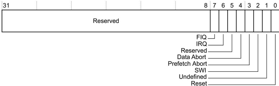
Figure 12-6 Vector Catch Register format
