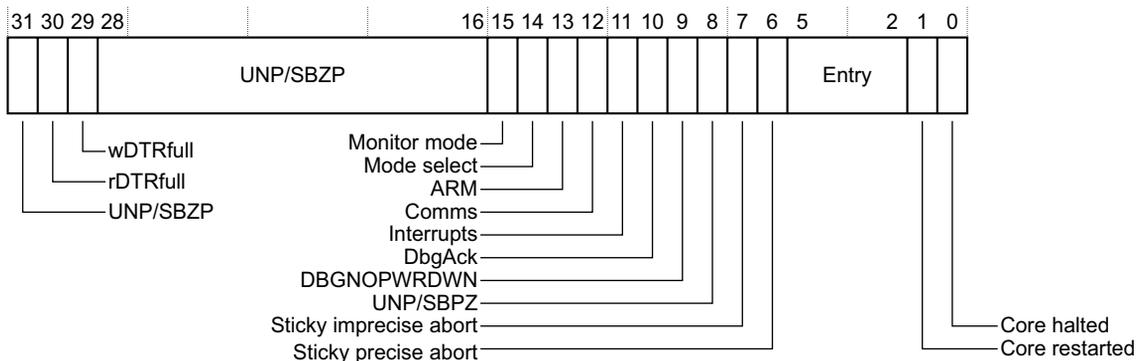
Figure 12-3 Debug Status and Control Register format
