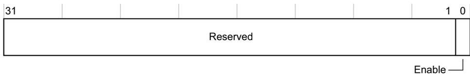
**Figure 10-2 Interrupt Distributor Control Register format**
