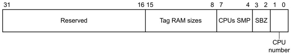
**Figure 9-2 SCU Configuration Register format**
