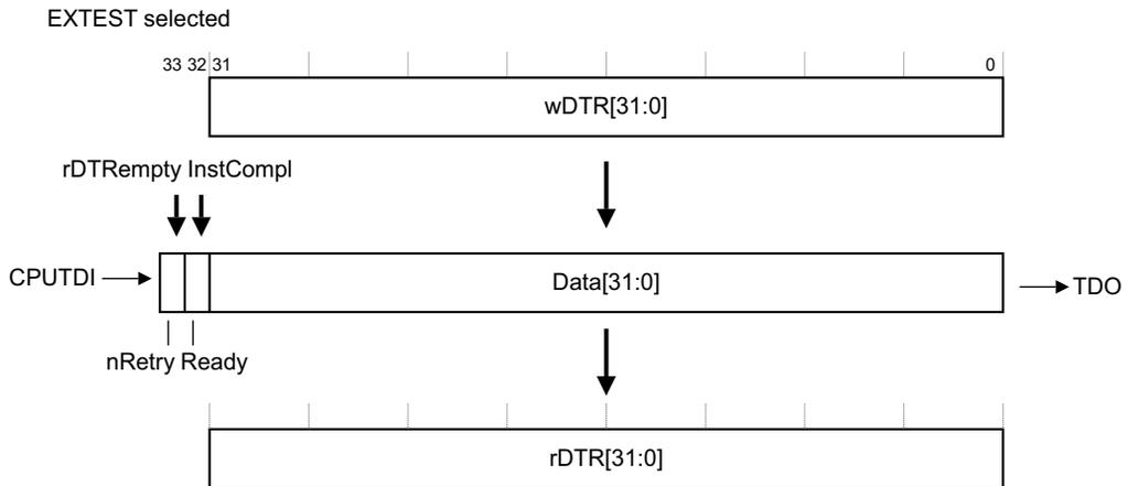
**Figure 13-9 Scan chain 5 bit order, EXTEST selected**
