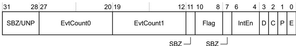
**Figure 3-41 Performance Monitor Control Register format**
