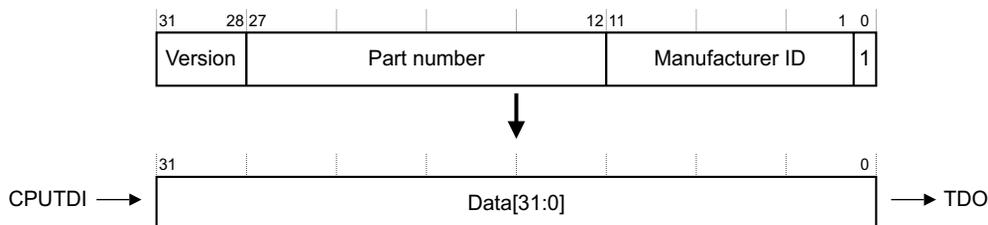
**Figure 13-3 Device ID code register bit order**
