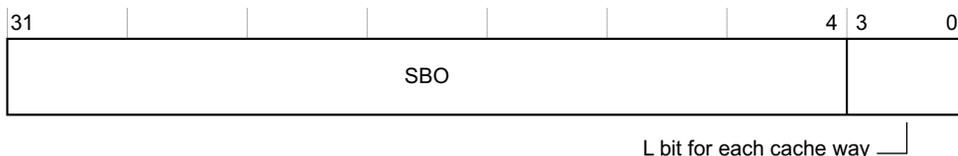
**Figure 3-35 Data Cache Lockdown Register format**
