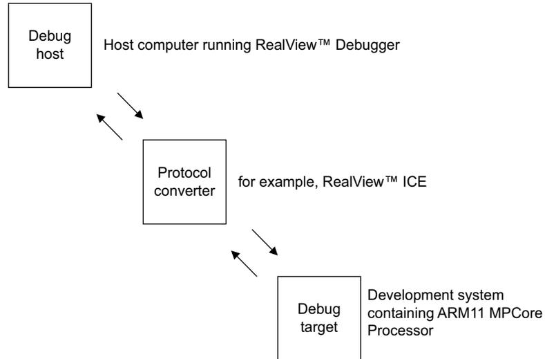
**Figure 12-1 Typical debug system**
