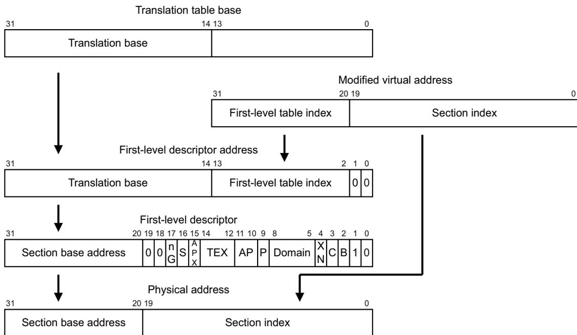
**Figure 5-11 Translation for a 1MB section, ARMv6 format**
