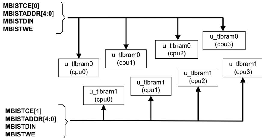
Figure C-7 TLB RAM organization with four MP11 CPUs
