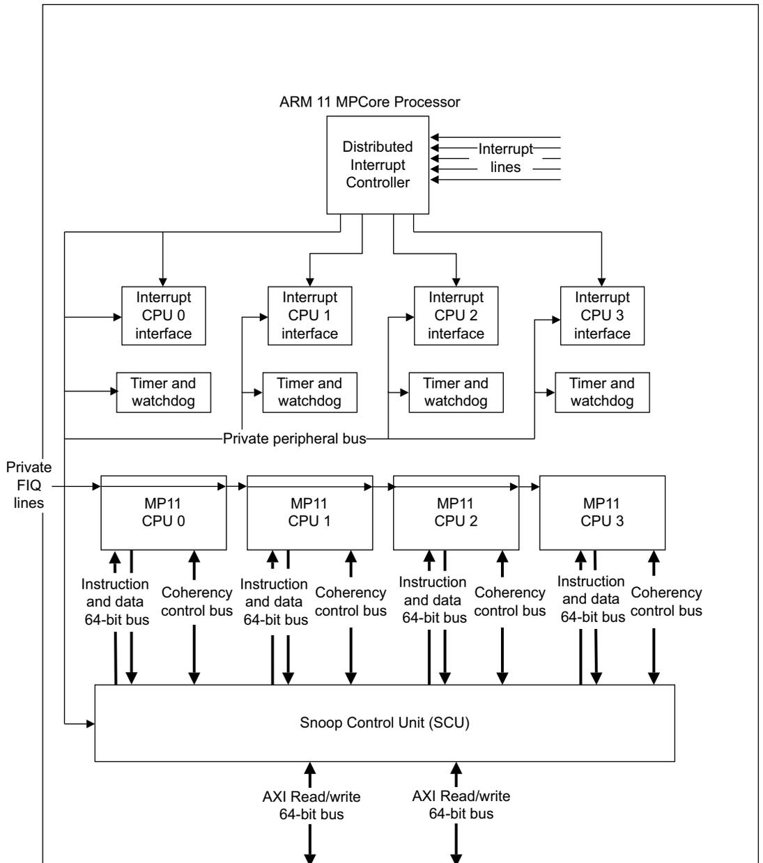
Figure 1-1 ARM11 MPCore processor block diagram
