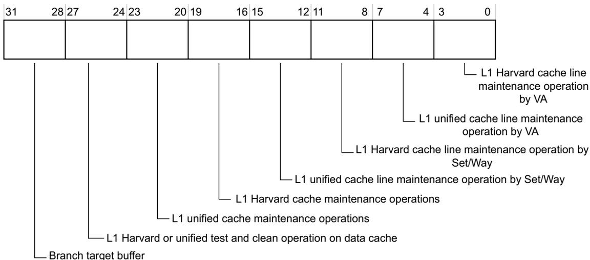
**Figure 3-10 Memory Model Feature Register 1 format**
