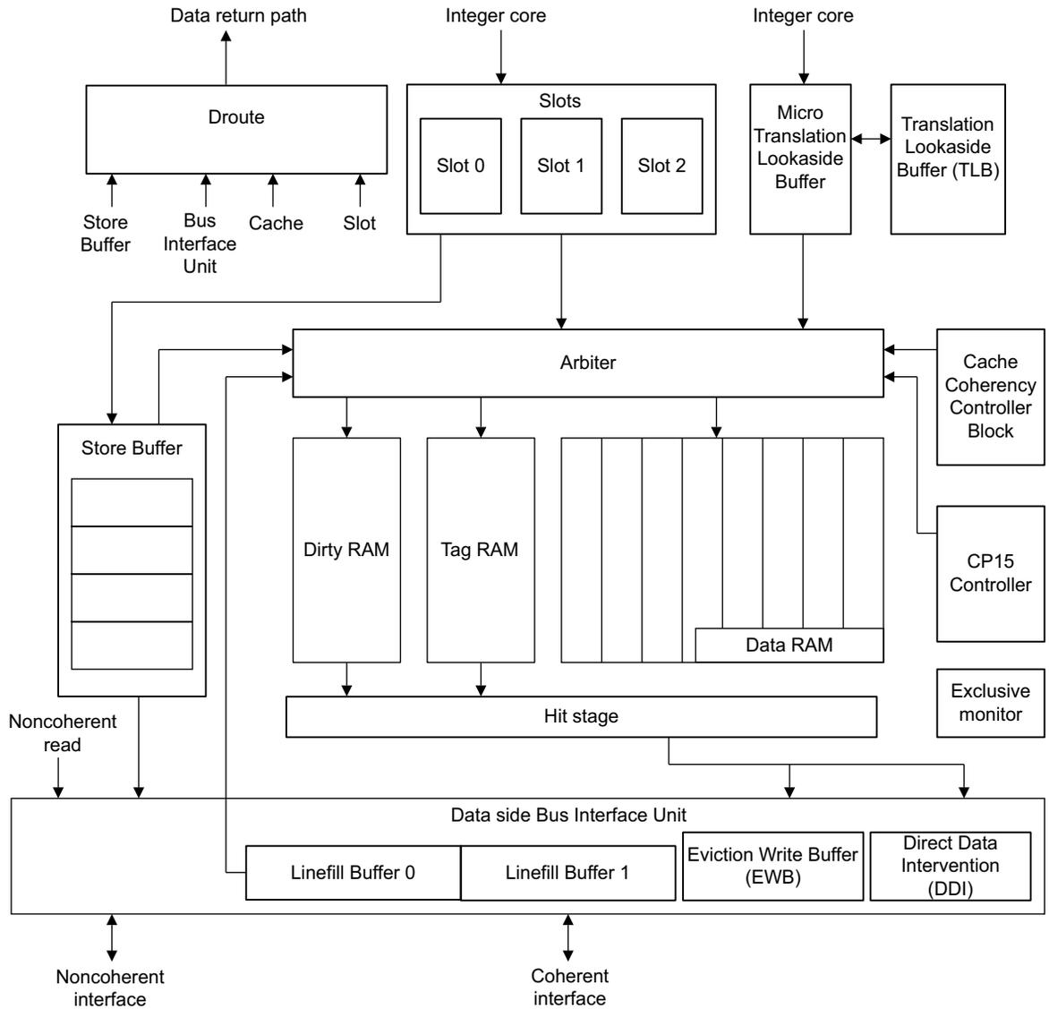
Figure 7-1 Level 1 data side memory system block diagram
