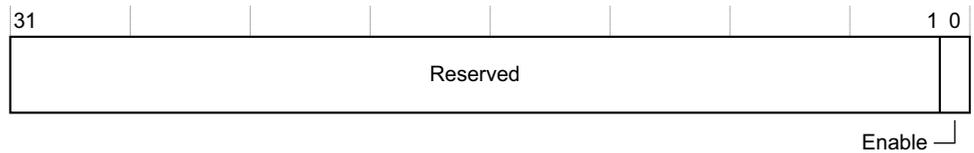
**Figure 10-8 CPU Interface Control Register format**
