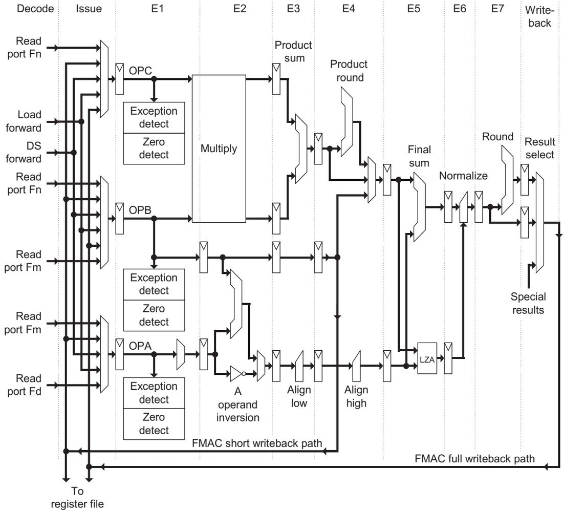
Figure 16-1 FMAC pipeline
