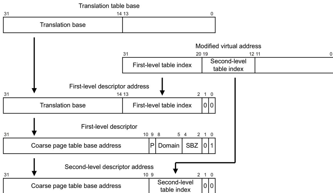
**Figure 5-13 Generating a second-level page table address**
