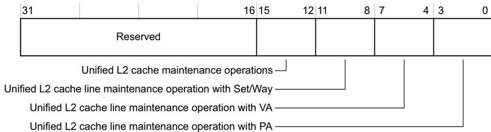
**Figure 3-12 Memory Model Feature Register 3 format**
