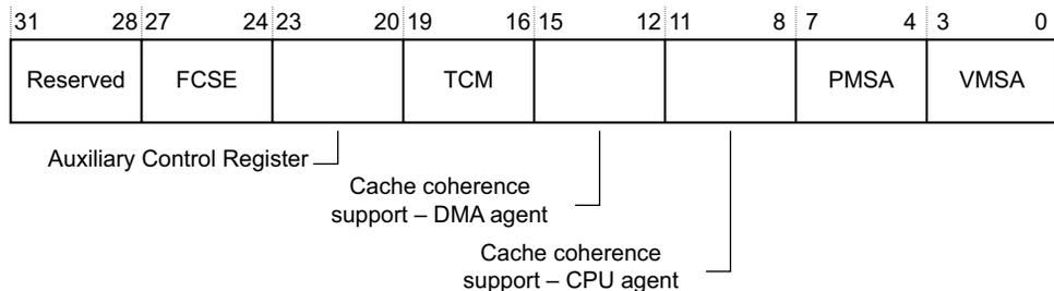
**Figure 3-9 Memory Model Feature Register 0 format**
