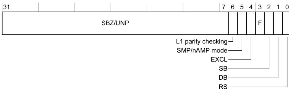
**Figure 3-19 Auxiliary Control Register format**
