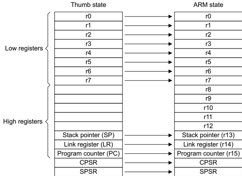
**Figure 2-6 ARM state and Thumb state registers relationship**
