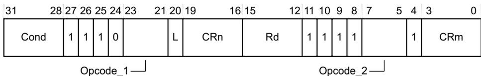
**Figure 3-1 CP15 MRC and MCR bit pattern**
