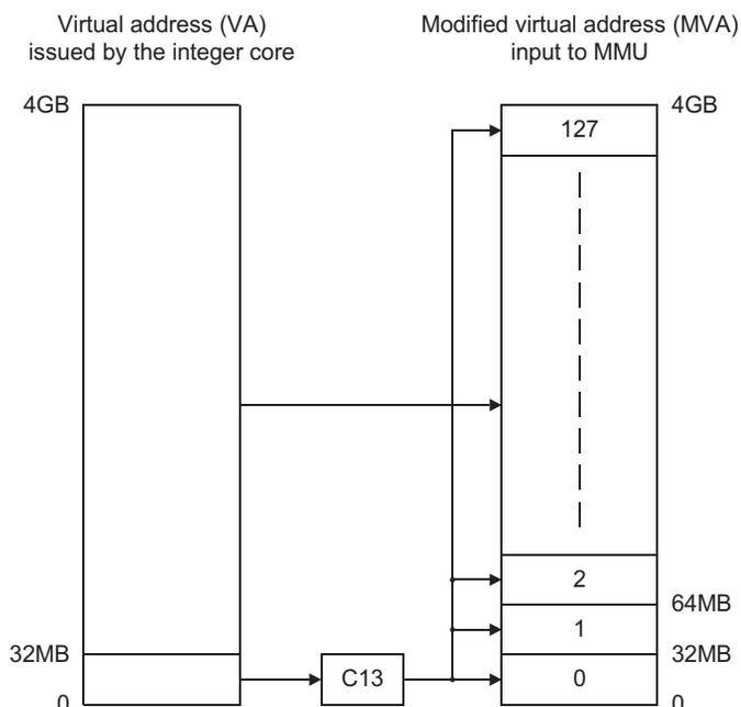
**Figure 3-38 Address mapping using CP15 c13**
