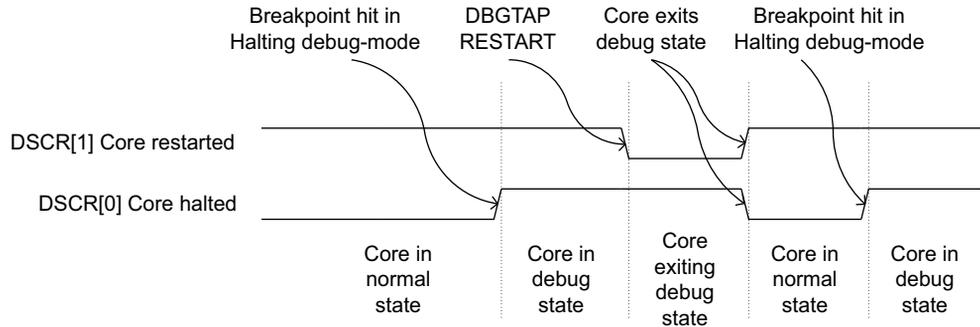
**Figure 12-4 Core restarted bit and core halted bit**
