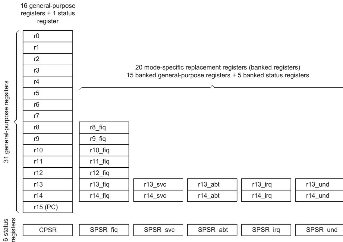
Figure 2-4 MPCore register set showing banked registers
