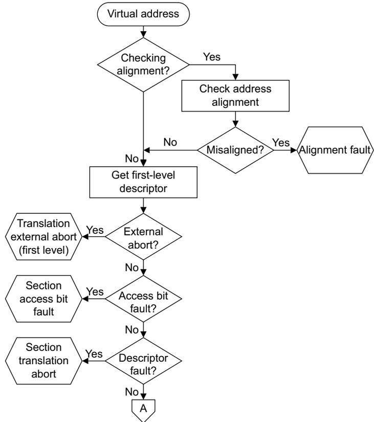
**Figure 5-1 Translation table managed TLB fault checking sequence 1**
