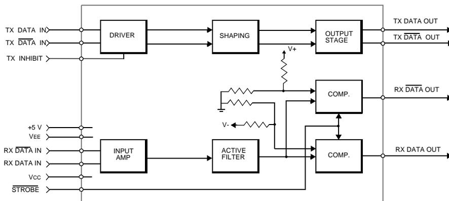
Block Diagram (without Transformer), 1/2 of unit shown
