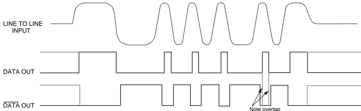
NOTE: Waveforms shown are for normally low devices. For normally high receiver output level devices, the receiver outputs are swapped as shown by the dashed lines
