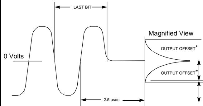
\*Offset measured at point A-A' in Fig 5
