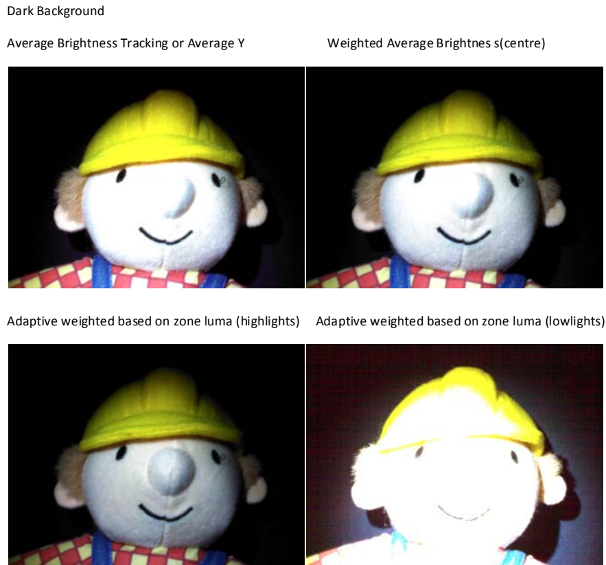
Figure 35: Using Adaptive Weighted AE for Highlights
