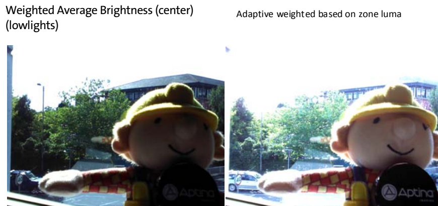
Figure 34: Advantage of Using the Adaptive Weighted AE
