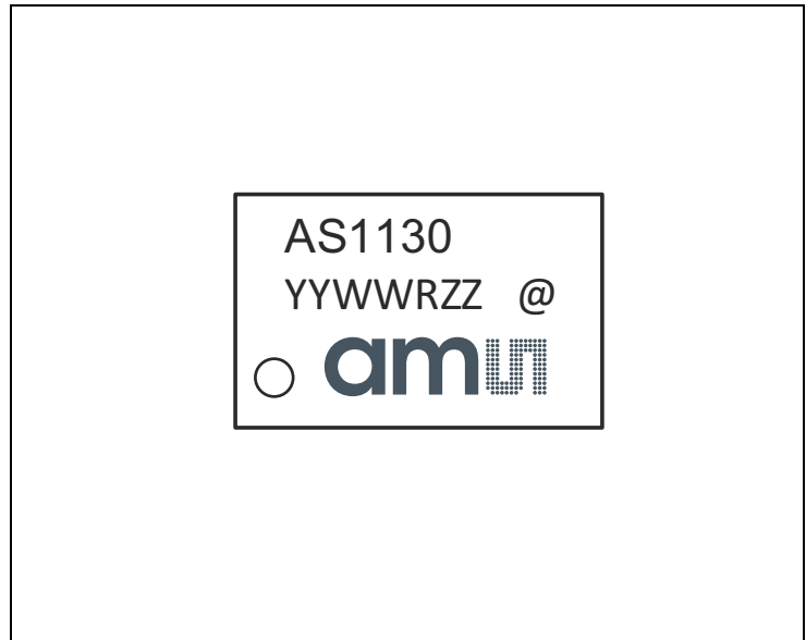
Figure 63: 28-Pin TSSOP Marking
