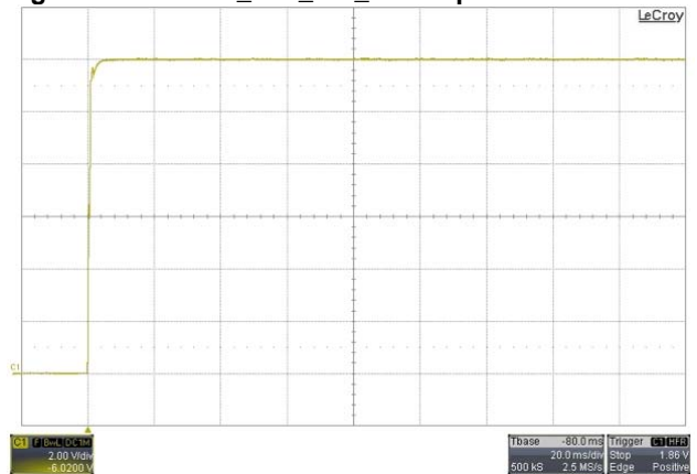
Figure 7 - Vin=57V 12V 3A Start Up
