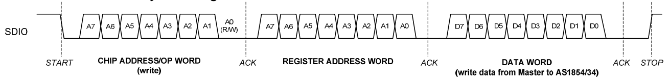
Figure 29 - I 2 C Interface Write Cycle Timing
