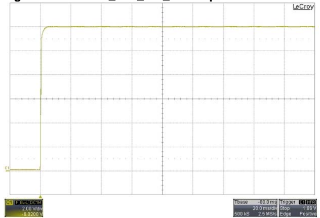
Figure 5 - Vin=48V 12V 3A Start Up with el load
