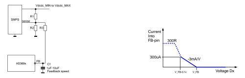
The characteristic of the feedback function can be seen in the diagram. The final output voltage of is determined by the setting of VFB and the current that is drawn from the external voltage divider.
