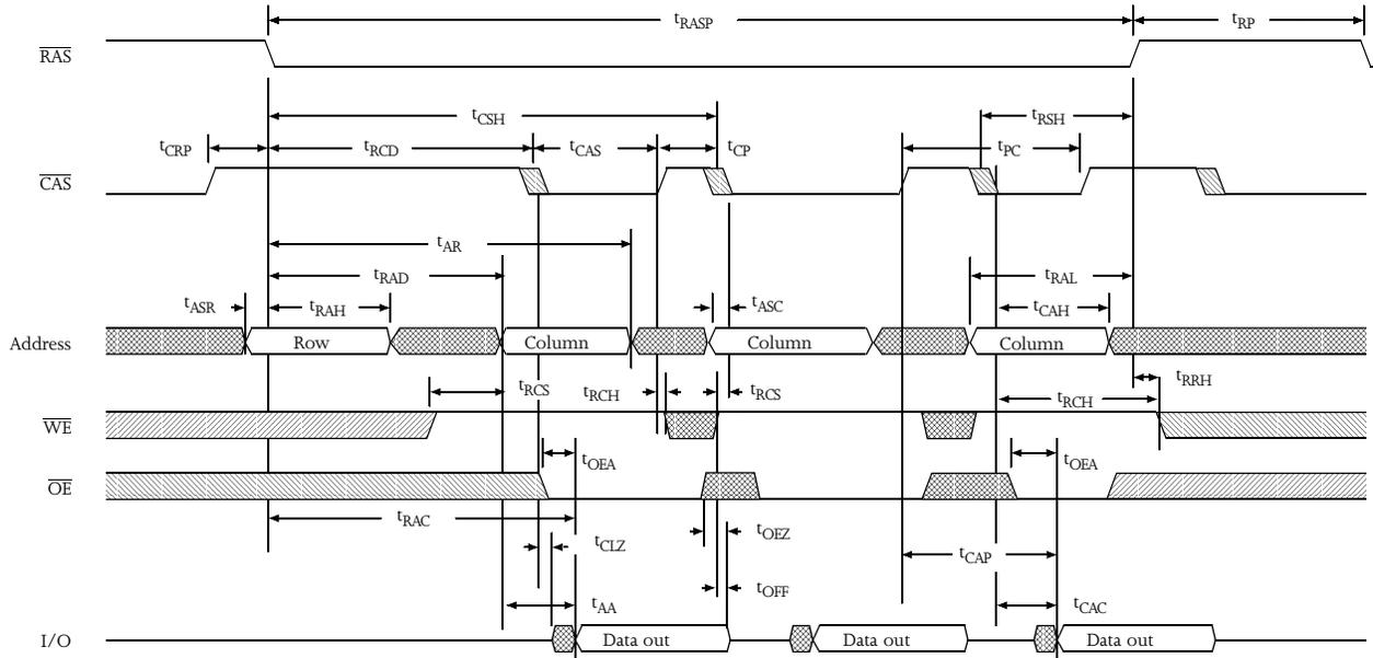
Fast page mode byte write waveform
