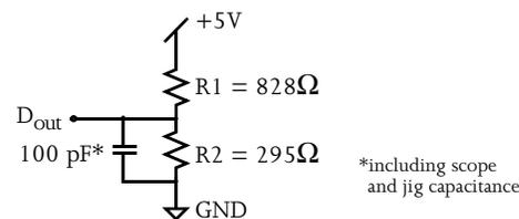
Figure A: Equivalent output load
