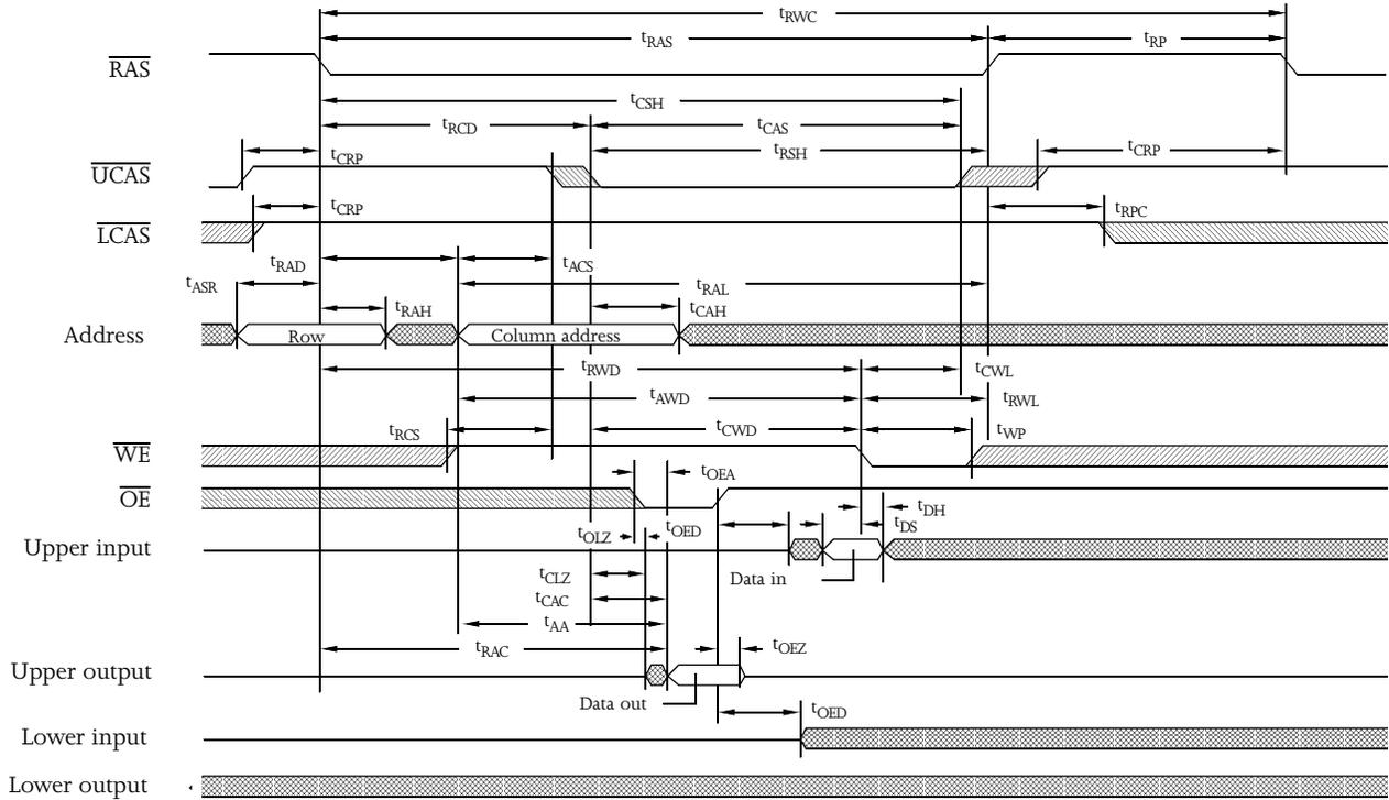
Lower byte read-modify-write waveform
